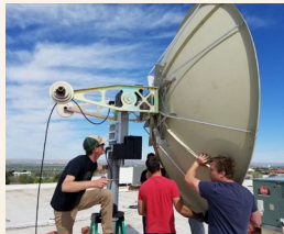
Student's Assembling 3m Dish System
